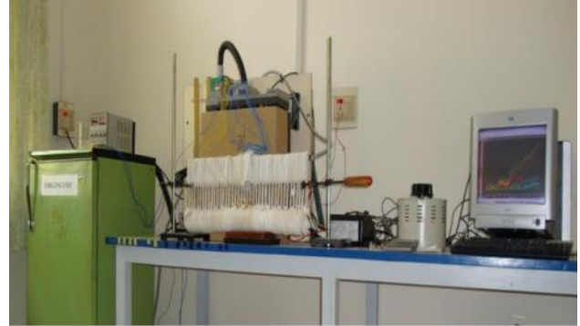
Experimental facility for closed loop pulsating heat pipe
