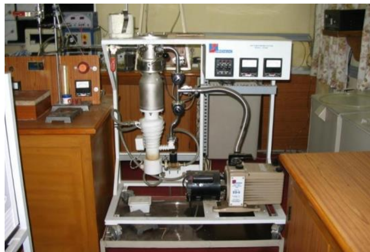
Vacuum Pumping Facility
