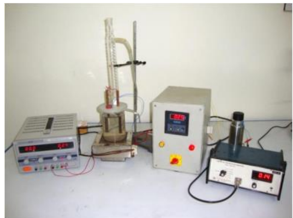
Experimental facility for pool boiling heat transfer
