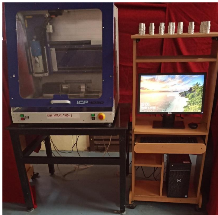
Fig. 6 CNC 4-AXIS MILLING / DRILLING TRAINER
