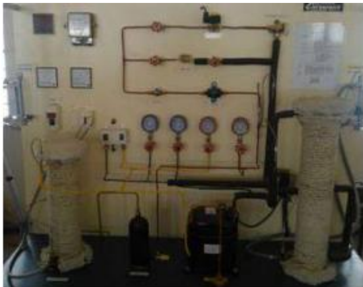
Fig. 6 Heat Pump Equipment
