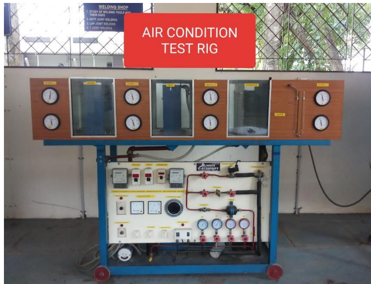
Fig. 4 Air conditioning Equipment
